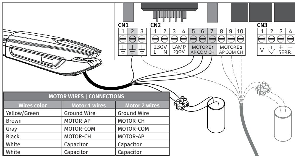
Connections should be made as shown above, connecting the 6 motor wires to the appropriate inputs of the control board and capacitor.
