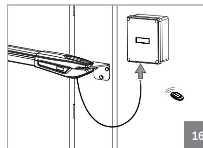
**04 • Connect the automation to the control board and configure the control devices.**
