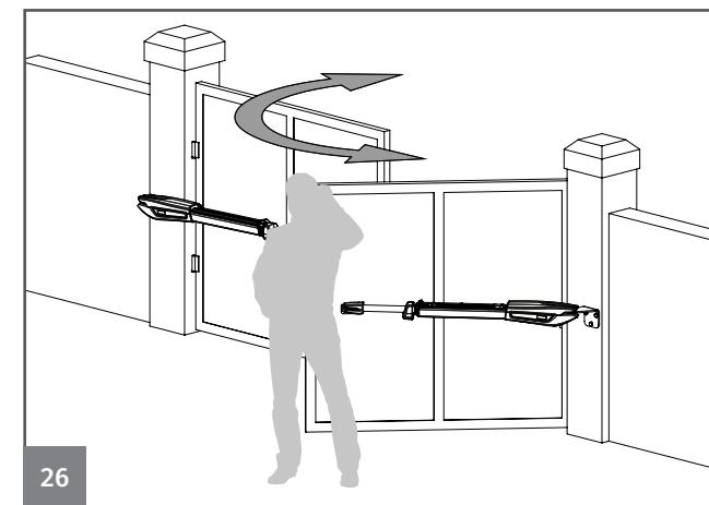
09 • Test the gate manually and if necessary readjust the micros, as indicated in the previous paragraphs.
