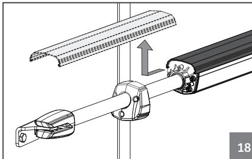
02 • Loosen the 3 front screws, remove the cover and the profile cover.
