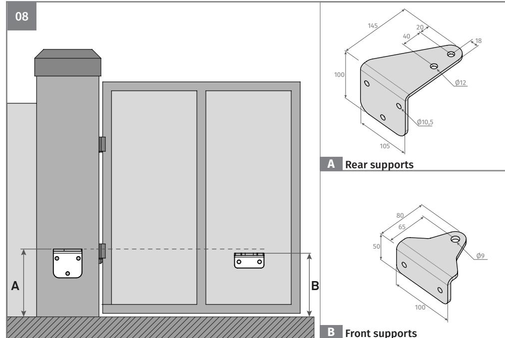
Dimension A • Vertical distance from the floor to the top of the rear support.
