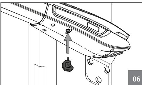
Place the unlocking key in the slot signed on image 05 (motor installed on the left) or 06 (motor installed on the right).
