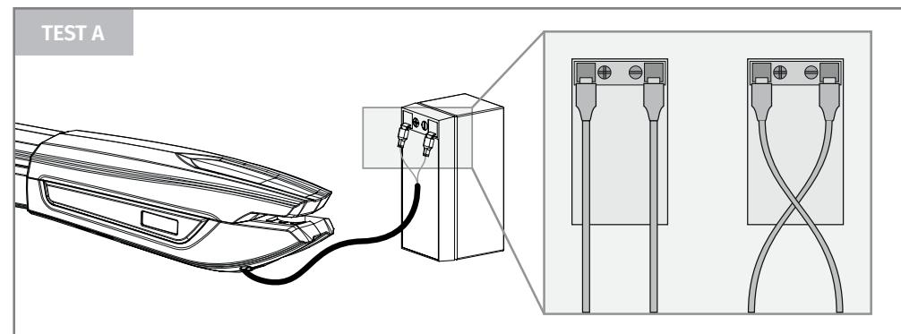
**Test A** • Make the connections as indicated in the image. If the motor works, the problem is in the control board. If it does not operate, do the test B.
