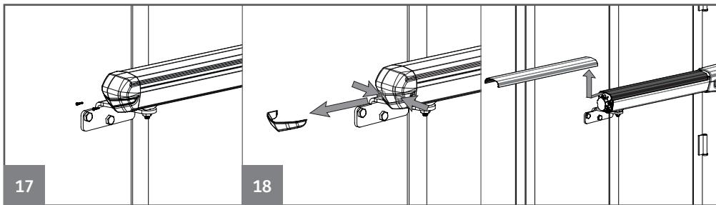
02 • Remove the chrome clip with a screwdriver.
