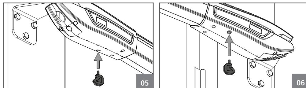
Place the unlocking key in the slot signed on image 05 (motor installed on the left) or 06 (motor installed on the right).
