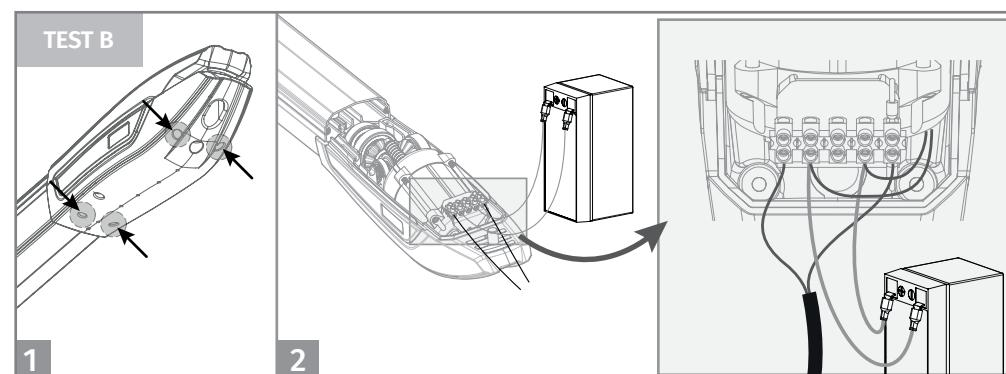
**Test B** • Loosen the 4 screws to remove the cover and access the internal connections. Make the connections as indicated in the image. If the motor works, the problem is on the diode(s) or on the micro(s). If it does not operate, replace with a new 24V motor and re-test to ensure that all is ok.
