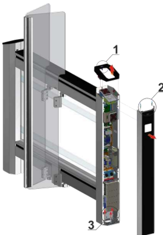
Fig. 13 – Turnstile dismantling and remove from pallet
