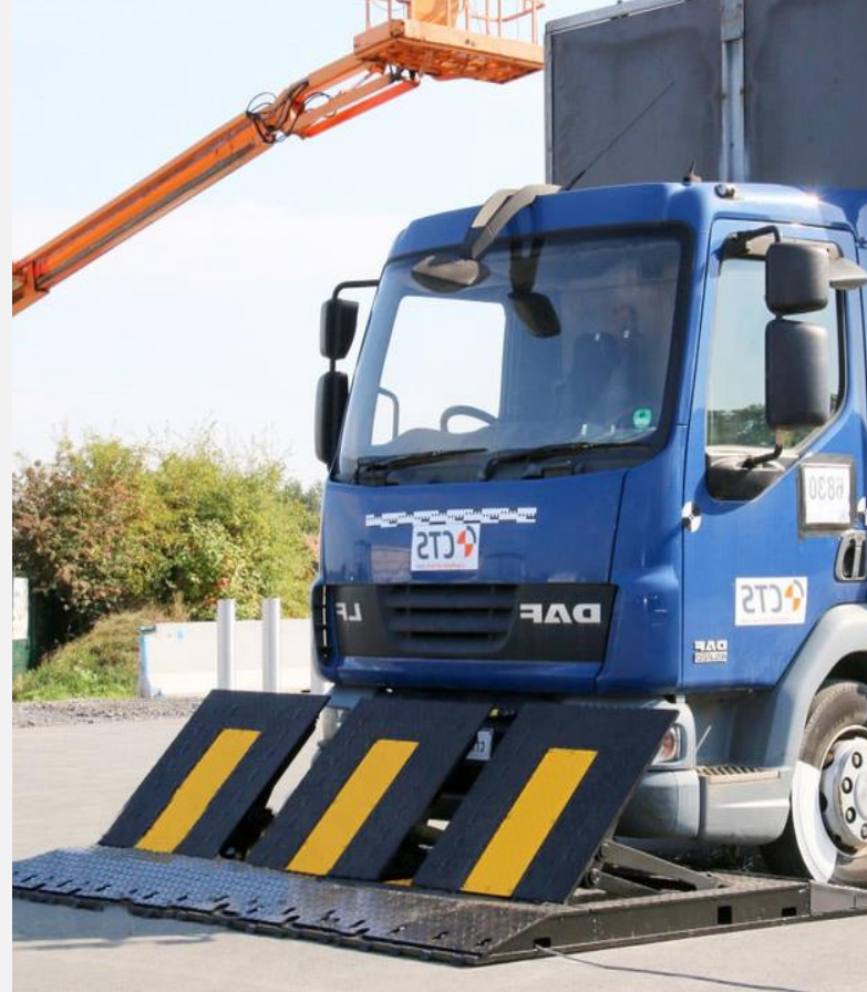
On the photo is a TiSO Mobile Speedbump (road blocker) during testing for the IWA 14-1 standard. The crash test was successful; the road blocker has confirmed its protective properties.
