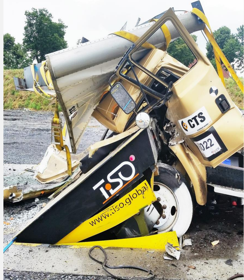
On the photo is a TISO road blocker during testing for the ASTM F2656 standard. The crash test was successful; the road blocker has confirmed its protective properties.
