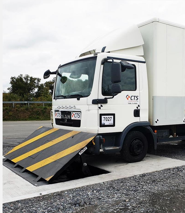
On the photo is a TiSO road blocker during testing for the PAS 68:2013 standard. The crash test was successful; the road blocker has confirmed its protective properties.
