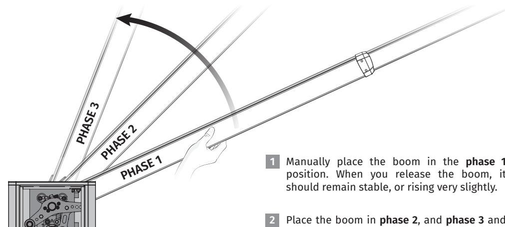
1 Manually place the boom in the **phase 1** position. When you release the boom, it should remain stable, or rising very slightly.
