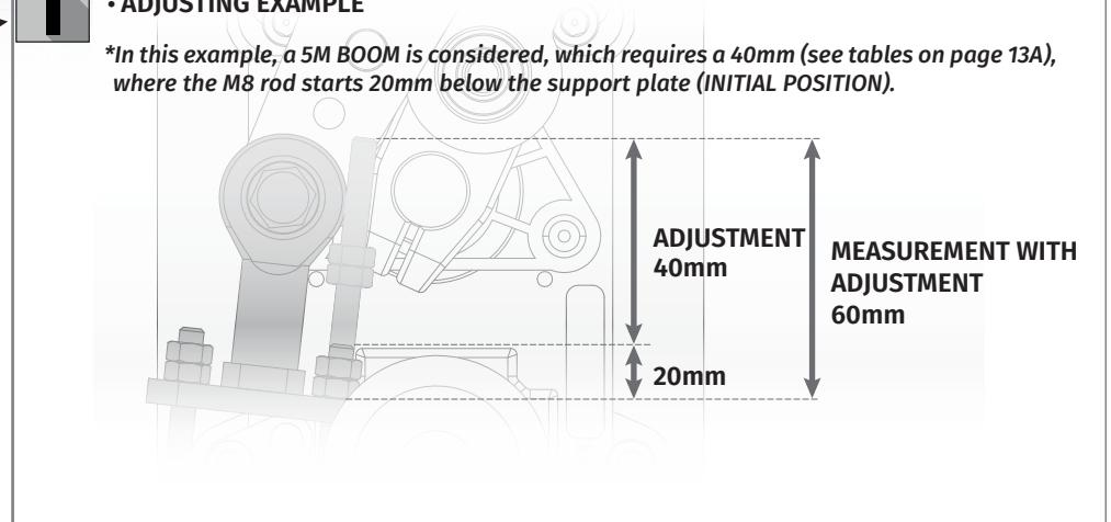
**4** Hold the threaded rod with pliers to prevent it from rotating, and tighten the adjusting nut until the spring is stretched to the distance mentioned in the table on page 13A.
