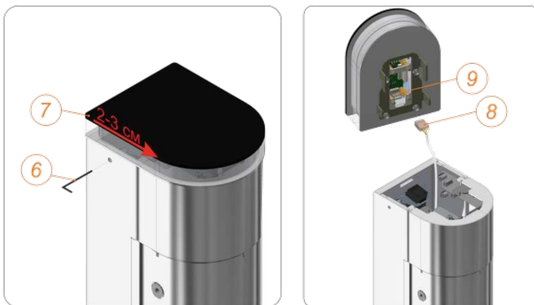
Fig.18 – Installation of the top cover on the turnstile rack
